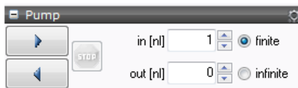
Figure 6.19: Set the pump volumes and launches pumping by pressing Pump in or Pump out
