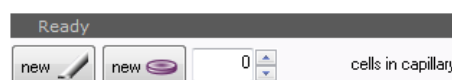
Figure 6.16: The status panel summarizes the calibration status of the of the mmi CellEctor. If a calibration is pending "calibration pending" will be displayed in the header.
